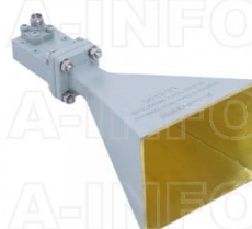
LB-42-20-C-SF Standard Gain Horn Antenna 18-26.5GHz 20dB Gain SMA Female
